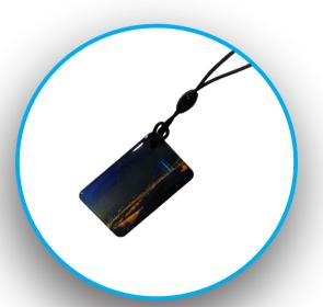
They are the key fobs that are used in the entrance doors of the apartments, offices, buildings, instead of using a key, which allow the door to be opened when it is closer to the smart lock on the door.
